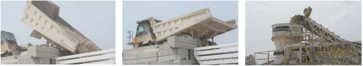
Figure 18. Large pieces of limestone are hauled by truck to a crusher, where they are crushed into smaller pieces. Most of the crushed rock is used as a base layer for road construction.
