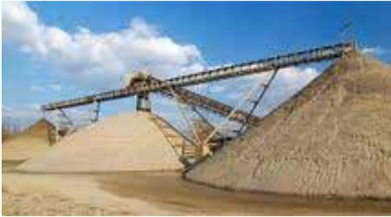
Figure 16. Gravel stockpiles are stored according to particle size
